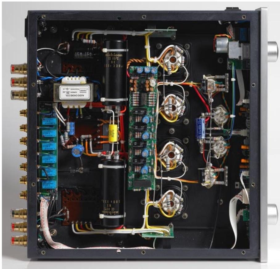
The DiaLogue Two is hand-made and point to point wired although it does contain a couple of internal printed circuit boards, one notably for the unique "Adaptive AutoBias" circuit, which is claimed to optimize valve performance and reduce distortion by 40 to 50%. It also extends tube life and makes the unit more reliable and user-friendly.
