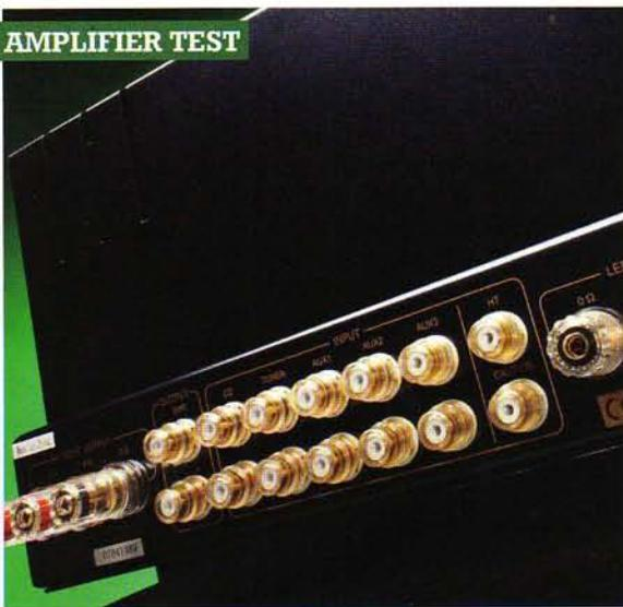
ABOVE: On the rear of the amp can be found five line-ins, a tape loop, a home theatre input that bypasses the preamp section, plus 4 and 8ohm speaker taps
