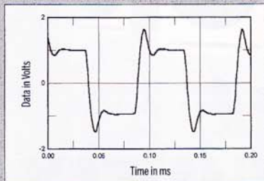
Fig.3 PrimaLuna DiaLogue Premium HP, 8 ohm tap, ultralinear mode, small-signal 10kHz squarewave into 8 ohms.
