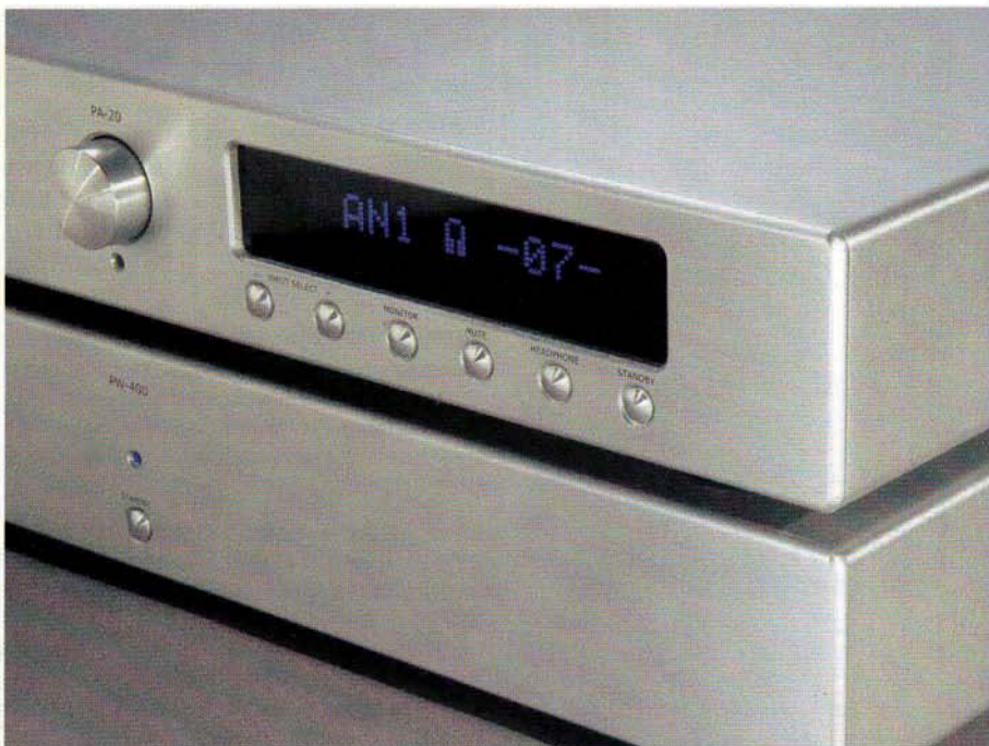
RIGHT: The PA-20 preamp's volume control offers independent line/headphone output and adjusts in larger or finer steps according to how fast you spin the dial. Volume, input selection, tape monitor and mute are also on the remote
